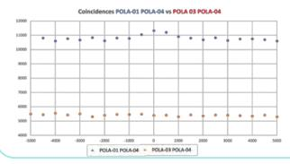
The plots show the distribution of difference of arrival time of muons in the POLA-01 POLA-04 (upper left) and the POLA-03 POLA-04 (upper right); from the plot it is clear that as the distance between detectors increase the coincidence peak is less visible over the background, as expected (left)
