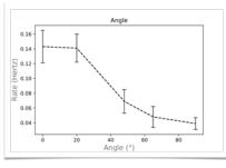
Larger angles yield lower rates, where 0° indicates a vertical measurement and 90° denotes a horizontal measurement.
