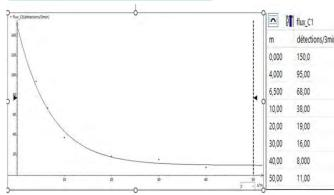
On the water surface we detected 50 muons/min and 4,7 muons/min at 50m depth. Flow is divided by 2 every 5m with 15 % incertitudes.
