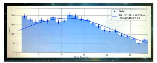
Muons detected show a peak of events at 11.24 ns, which results in a calculated velocity of:  $v = \frac{s}{t} = \frac{3,19 m}{11,24 \cdot 10^{-9} s} = 283,807,829.2 \frac{m}{s} = 0.95c.$
