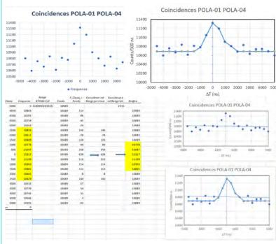
The graphs show the coincidences between POLA-01 and POLA-04. The peak is found at the frequency of 11137, with 628 coincidences in the class range.
