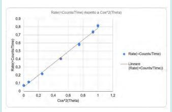
In figure: the graph obtained from data elaboration of the experimental data, which shows the expected relation on cos<sup>2</sup>(theta) of the count rate
