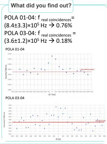
Our analysis confirmed that the frequency of real coincidences decreases exponentially with the distance between the couple of detectors .
