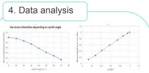
We find that when the detector area and the distance between the detectors are determined, as the Angle of the muon telescope increases, the number of muon per unit time is measured by the detector decreases.There's a nice linear relationship between f and  $(\cos\theta)^2$ .
