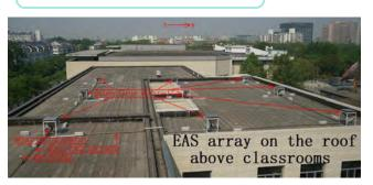
On the roof of Dongzhimen Middle School, a detector array is built to measure Extensive Air Shower (EAS), as shown in the above figure.
