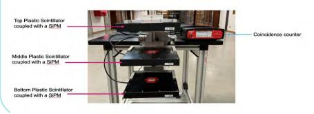
We have used three different layers so that we can get very precise data and understand if the signal is generated by a muon.
