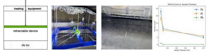
Fig.1 Diagram of our cloud chamber Fig.2 Photograph of cloud chamber Fig.3 An observed electron track
