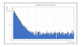
The free muon decay lifetime has been determined to be:  $\tau = 2,2$  ms.
