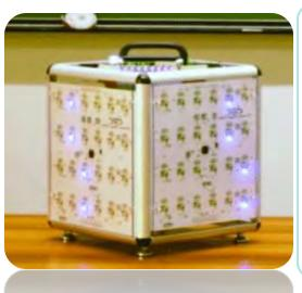
Finally we used the cosmic cube in our experiment. This tool is specifically designed to the muon flux. It consists of 4 layers each one provided with 6 rods of plastic scintillators which detect the passage of particles and light up. We know that muons are the only particles able to penetrate the 4 layers of the tool and so the only particle to be analyzed via the CRC
