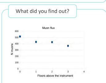
This graphic represents the muon rate in function of the number of floors over the instrument. The number of floors changes significantly the rate.
