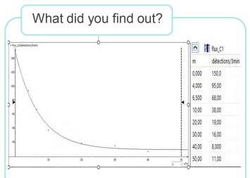
On the water surface we detected 50 muons/min and 4,7 muons/min at 50m depth. Flow is divided by 2 every 5m with 15 % incertitudes.
